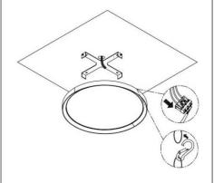
1.Connect the ceiling AC wire to the plate terminal, wiring method: (L-live wire) (N-neutral wire) (-ground wire)
