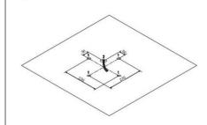
First select the place to be installed, place the ceiling bracket in the mounting position, and mark it with a pen core
