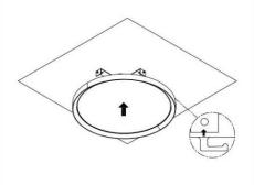
Lift the frame of the lamp and align the four notches with the four installation pillars of the ceiling bracket.
