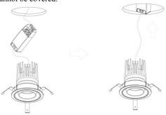
5. Fold up the three shrapnel of the downlight, then install the downlight to the hole as shown to make sure the downlight cannot fall off.
