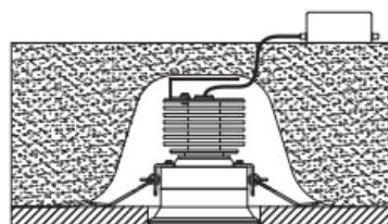
Driver must be installed above insulation.
