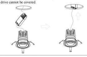
5. Fold up the three shrapnel of the downlight, then install the downlight to the hole as shown to make sure the downlight cannot fall off.
