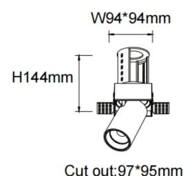
Real luminous flux (Lm) 3000 Luminous efficiency (Lm/W) 100 Beam angle (º) Life time (h) 50000 h L80B10 Colour **Black** Control gear included **Control** gear **Dimmable Casamby ready** Flicker Free Yes Light source **LED** Type of LED СОВ 3000 Colour temperature (K) Colour consistency (SDCM) SDCM<3
