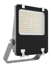
Lavov flood light from the family AQUILA II with a power of 100W and an optics 26x60° tilt10° degrees . CCT 4000K. With a total lumen output of 15500lm and a luminous efficiency of 155lm/W.DALI driver. Made in die cast aluminum and finished in Black color. IP66 and IK 08 degree of protection.
