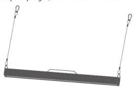
2. Suspended Installation: Making clasp, rings and lifting rope fixed successively on high bay and then hanging the other end of lifting rope in right place like below picture.
