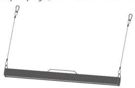
2. Suspended Installation: Making clasp, rings and lifting rope fixed successively on high bay and then hanging the other end of lifting rope in right place like below picture.
