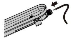
3.Insert the cable through the cable gland
