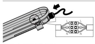
4. Connect the wires to the wiring terminal
