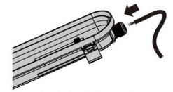
3.Insert the cable through the cable gland
