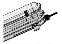
6. Put back the LED module and diffuser
