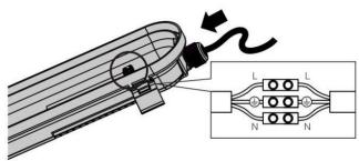
4. Connect the wires to the wiring terminal
