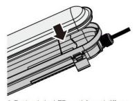
6. Put back the LED module and diffuser
