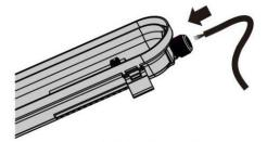
3.Insert the cable through the cable gland
