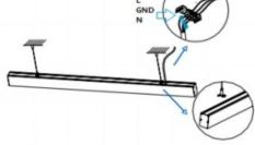
3.Connect the wire by junction box poweroff simultaneously.
