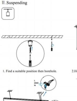
3.Connect the wire by junction box poweroff simultaneously.
