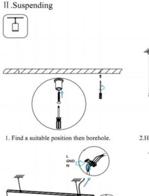
Connect the wire by junction box poweroff simultaneously.
