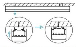
2.Put the snap-fit into the setscrews and lock it tightly.
