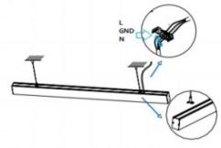
Connect the wire by junction box poweroff simultaneously.
