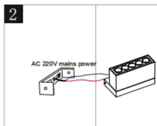
Connect the reserved power supply wire to the lighting fixture power wire
