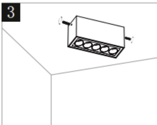
Use the screws provided with the fixture to secure the light to the ceiling.
