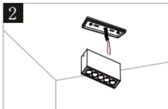
Connect the reserved wires to the lamp's power supply, then tighten the lamp to the ceiling mount. .
