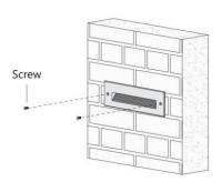
Install the light fixture on the wall
