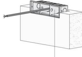
Insert support plates to prevent deformation of the recessed sleeve
