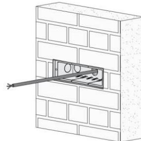
Finish the installation of concrete surface materials and remove the support plates
