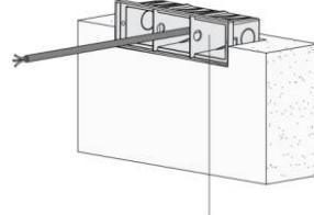
Insert support plates to prevent deformation of the recessed sleeve
