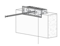
Insert support plates to prevent deformation of the recessed sleeve
