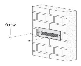
Install the light fixture on the wall
