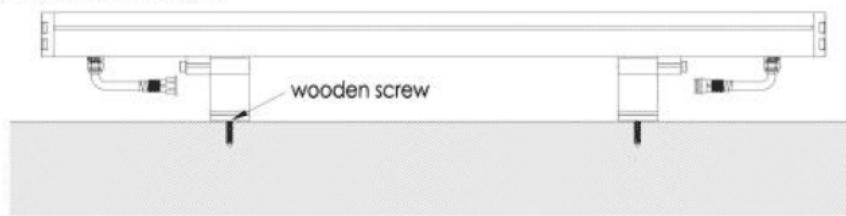
2. Loosen the M3 machine screws, adjust the distance between the two supports, and then lock the screws
