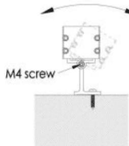
5、Loosen the M4 cup screw of the support, adjust the Angle of the lamp and then lock the screw
