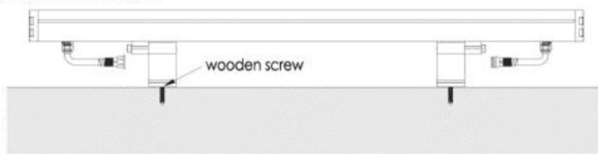
3. Attach the light fixture to the wall or floor with wood screws.
