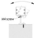
5. Loosen the M4 cup screw of the support, adjust the Angle of the lamp and then lock the screw
