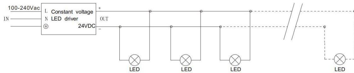
Explanations: the transmiss circuit of the whole group depends on the circuit of junction boxes. the max. current depends on the max. load of power cable between the junction boxes, but it is not related to the max. load current of power cable of the fitting. The outer dia meter of cable between the junction boxes is limited by the max. outer diameter of speedy plug, the max. allowed outer diameter is 10mm.
