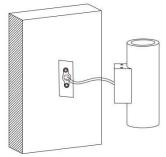
Connect the lighting fixture with the cable which is been prepared for the installation previously.
