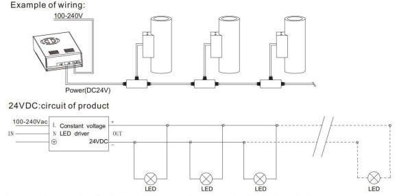
Explanations: the transmiss circuit of the whole group depends on the circuit of junction boxes. the max. current depends on the max. load of power cable between the junction boxer, but it is not related to the max. load current of power cable of the fitting. The outer dia meter of cable between the junction boxes is limited by the max. outer diameter of speedy plug, the max. allowed outer diameter is 10m m.
