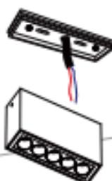
Connect the reserved wires to the lamp's power supply, then tighten the lamp to the ceiling mount.
