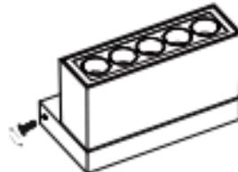
Use the screws provided with the fixture to secure the light to the ceiling.
