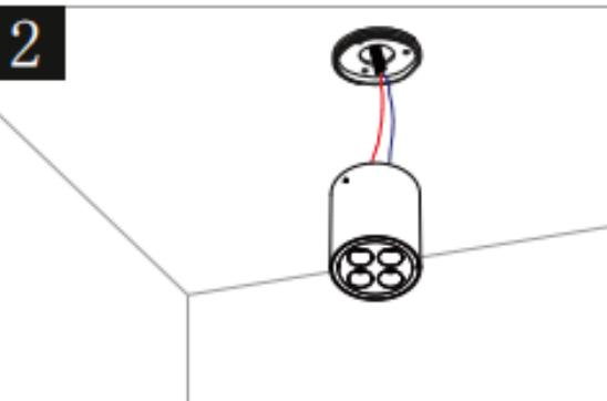
Connect the reserved wires to the lamp's power supply, then tighten the lamp to the ceiling mount..
