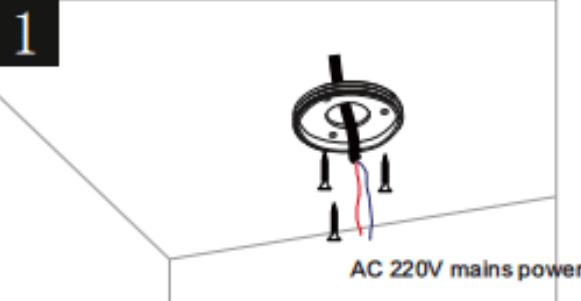
Attach the ceiling rose to the ceiling using the provided screws.
