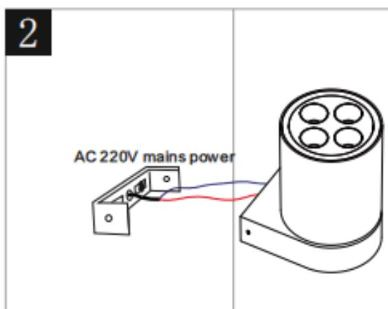
Connect the reserved power supply wire to the lighting fixture power wire
