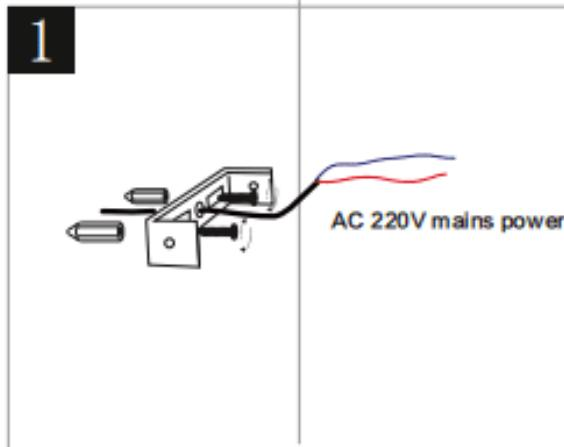
Install the mounting plate on the ceiling with the provided screws, leaving space for the power supply wires.
