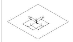
First select the place to be installed, place the ceiling bracket in the mounting position, and mark it with a pen core
