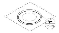
Rotate the frame of the lamp clockwise so that it locks into place with the ceiling bracket.
