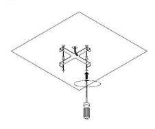
Take out 4 screws B and use a screwdriver to fix the ceiling bracket to the ceiling.
