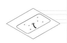
First select the place to be installed, place the ceiling bracket in the mounting position, and mark it with a pen core
