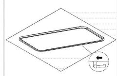
Rotate the frame of the lamp clockwise so that it locks into place with the ceiling bracket
