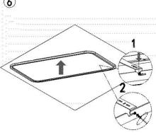
Lift the frame of the lamp and align the four notches with the four installation pillars of the ceiling bracket.
