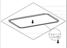
Make sure that the frame of the lamp is securely attached to the ceiling bracket.
