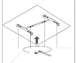
Take out 4 screws B and use a screwdriver to fix the ceiling
