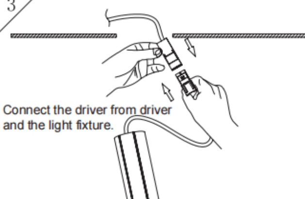
Connect the driver from driver and the light fixture.
