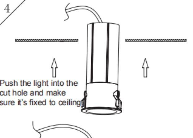
Push the light into the cut hole and make sure it's fixed to ceiling
