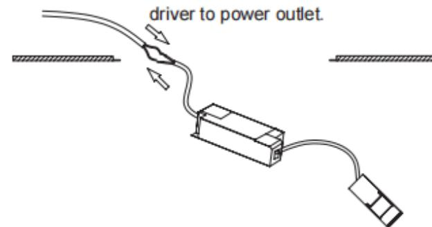
Connect the AC wire from driver to power outlet.
