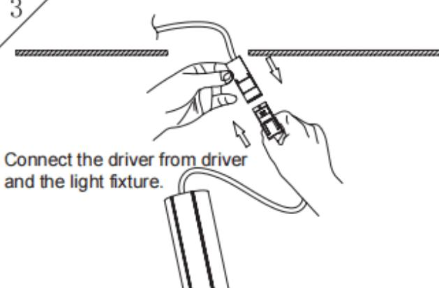
Connect the driver from driver and the light fixture.
