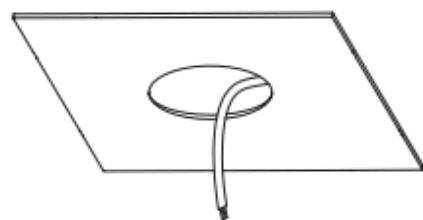
Made cut hole in ceiling accordingly to it's size and make wiring from the power outlet.
