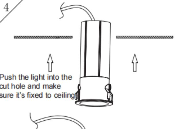
Push the light into the cut hole and make sure it's fixed to ceiling
