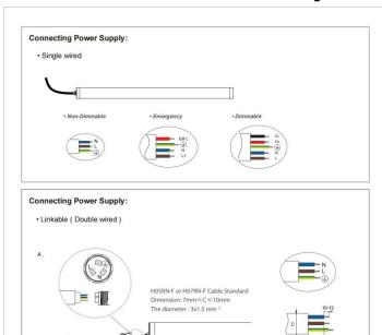
H05RN-F or H07RN-F Cable Standard Dimension: 10mm  $\leq$  C  $\leq$  14mm The diameter: 5x1.5 mm  $^2$
