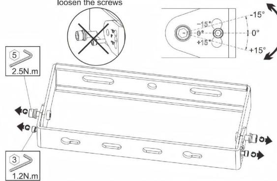
Fasten the M4 screws firstly, then the M6 screws
