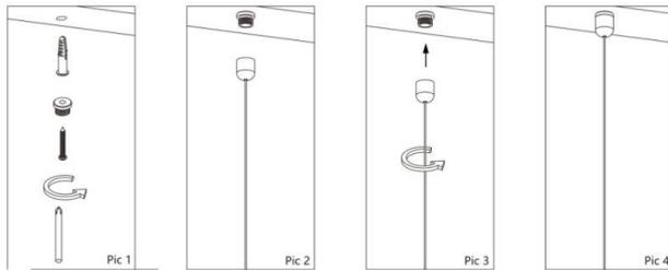
1. Drill plastic expansion pipe into ceiling, put the phillips screw through cylindrical bolt, then into expansion pipe, as diagrammatic deiction
