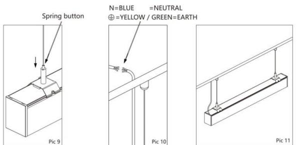
9. Connect the wire and buckle by pressing the spring button on the top of the lock nut, adjust wire length
