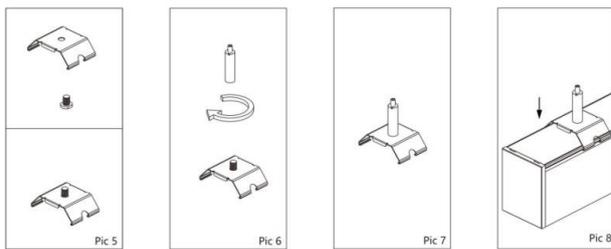
5. Put lock bolt through metal buckle, diagrammatic direction
