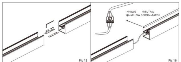
15. Connect lamps by connector, make sure both linear lights linked seamless, tighten the screws
