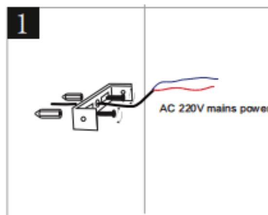
Install the mounting plate on the ceiling with the provided screws, leaving space for the power supply wires.
