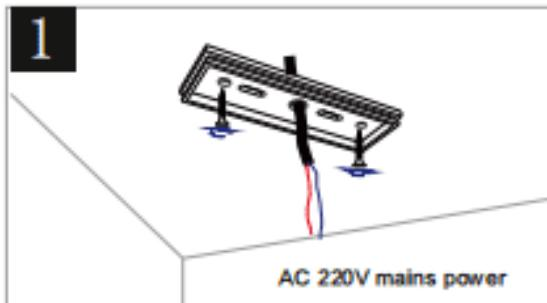
Attach the ceiling rose to the ceiling using the provided screws.
