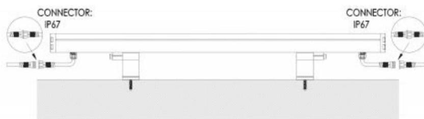
4、Align the power cable connector with the power cable connector of the lamp and connect it to the card position.
