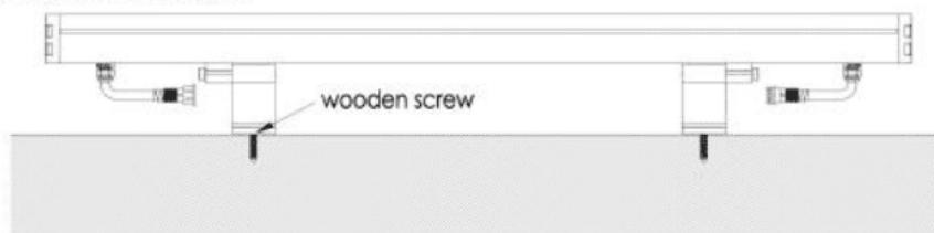
3、Attach the light fixture to the wall or floor with wood screws.
