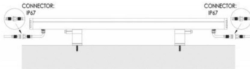
4、Align the power cable connector with the power cable connector of the lamp and connect it to the card position.
