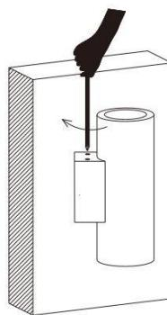
Fix the fixture on the back cover of the bracket with four screw
