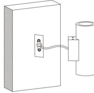
Connect the lighting fixture with the cable which is been prepared for the installation previously.
