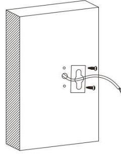
Fix the back cover of the bracket on the wall with two steel screw. Make sure the cable get through the hole in the middle of it.
