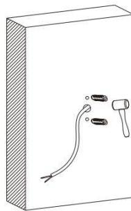
Drill two holes on the wall where you are about to install the lighting fixture. Then put two rubber plug into the holes respectively by using a hammer.
