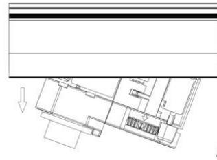
Remove the track adapter as shown
