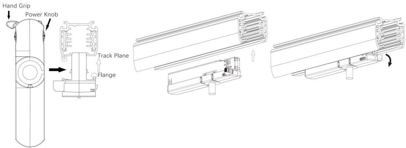
1. Make sure the track adapter's positions are the same as the picture showed before installation.
