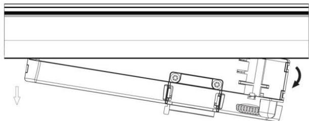
Remove the track adapter as shown
