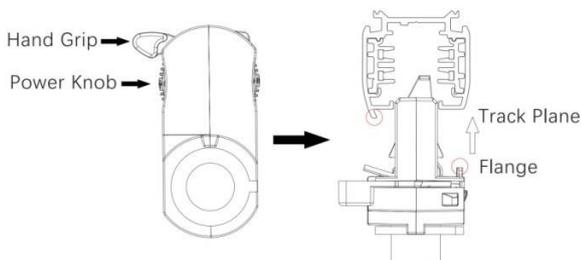
1. Make sure the track adapter's positions are the same as the picture showed before installation.
