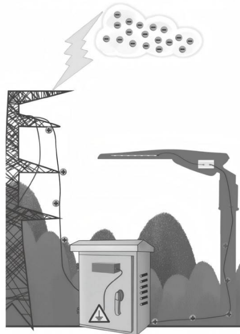
The SPD can absorb most surge energy before luminaire
